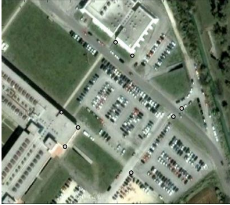
Figure 6.10: Deployment of the cameras (black circles) on the monitored environment. Each camera is placed at height 14m.
