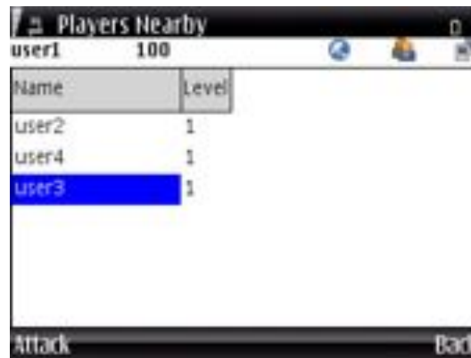
Figure 7.3: A screenshot of Geobashing showing the players in range. The three icons at the top right indicate (left to right) that GPS is online, players are in range and that the player is logged in.
