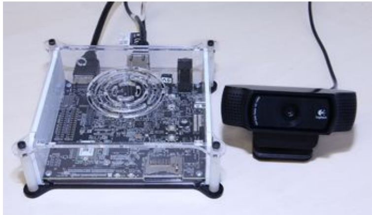
Figure 6.2: The PandaBoard based smart camera platform running Linux on a 1.0 GHz ARM processor with 802.11 b/g/n wireless connection interface. A Logitech C920 is used to acquire images with a native resolution of 3MP.
