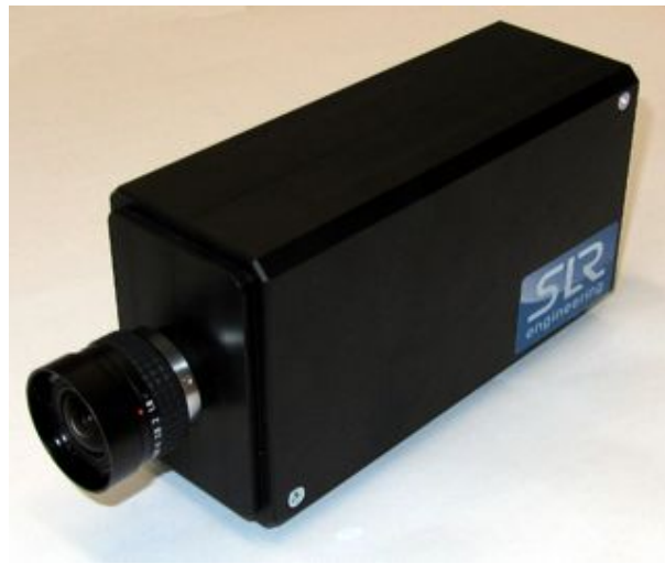
Figure 6.1: The SLR smart camera platform. A custom-built camera running Linux on a 1.6GHz Intel Atom processor with 2 GB memory and 100 MBit Ethernet interface. The image sensor is a CCD colour image sensor with a native resolution of 1280 \times 1024 pixels.
