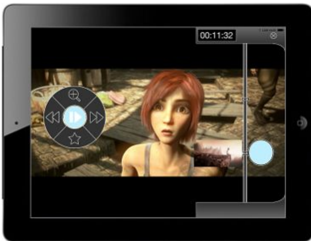
Figure 8.4: The default view of the initial version of the ThumbBrowser with its two main controls: a radial menu for the left thumb and a vertical seeker control for the right thumb.
