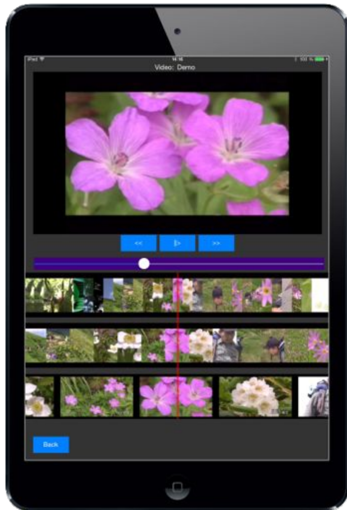
Figure 6.1: Interface of the KNT-Browser. Top: preview player window. Bottom: three shot-strips with different level of detail.
