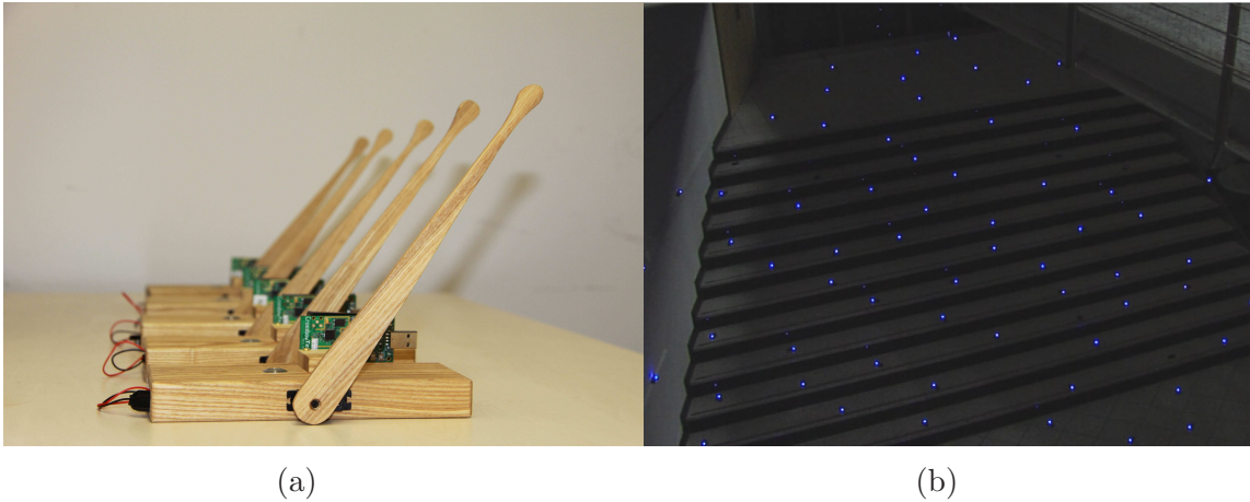
Figure 5.3: Snap shots of synchronization processes. In Panel a) we see TelosB devices attached to wooden pendula. The hands of the pendula show coinciding phase positions. In Panel b) we see Z1 devices distributed on a stairway. Some of these are already synchronized and show coinciding blue flashes.
