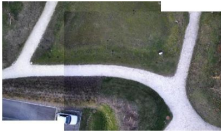
(b) Pixel-based registration between images 2 and 3. Different possible alignments are checked until the maximum correlation is achieved.
