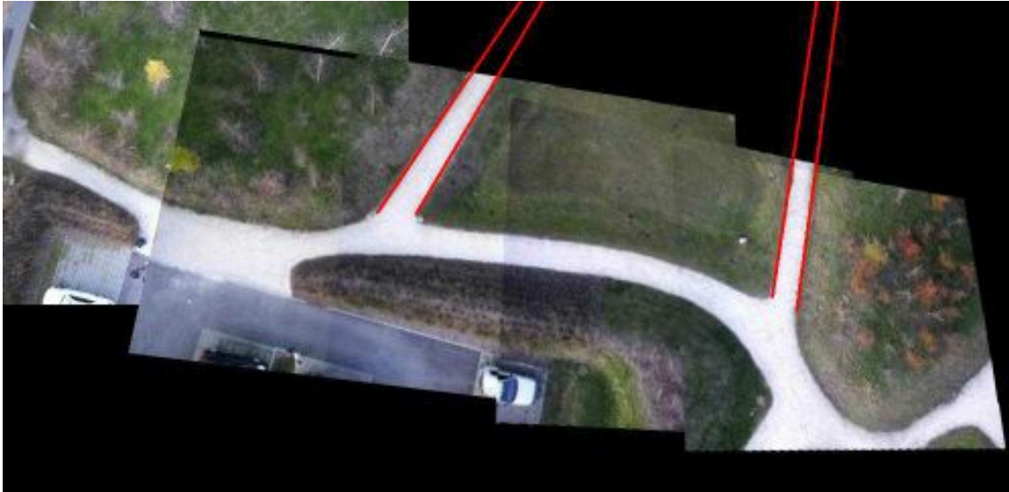
Figure 3.1: Mosaicking five images using SURF features. The path borders (red lines) are supposed to be almost parallel. This type of error accumulates over multiple images if not compensated.
