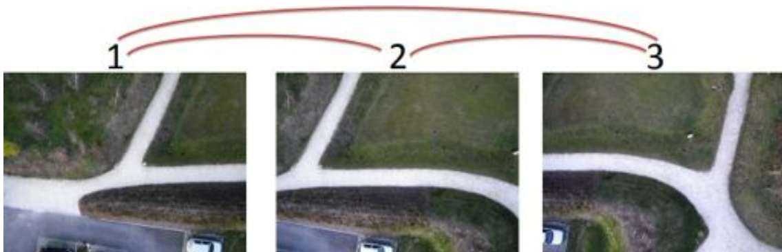
Figure 2.2: Sample three images to be mosaicked. In adjacency graph shown in red, images are the vertices and adjacent images are connected with an edge.
