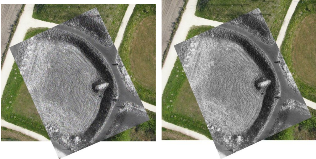
(c) Registered after homography of raw (distorted) images.
