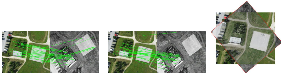
(a) SIFT features with 43 scale levels and Euclidean distance threshold 1.2 for matching. (b) SURF features with sampling step 1 and initial lobe 1. (c) Alignment and fusion.
