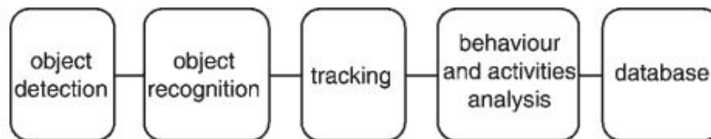
Figure 2.1: Traditional flow of processing in visual surveillance system. [3].
